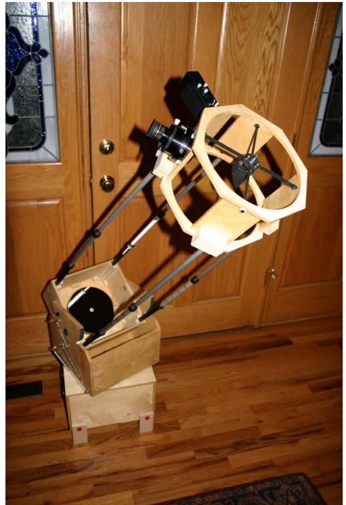
Initial use showed the scope to be top-heavy. Greg wished to avoid weighing down the box with counterweights. He applied the spring counterweight concept of Tom Krajci, modified for the small scope. Greg came up with novel spring routing which functions very well. Transport to Australia came off without a hitch.
