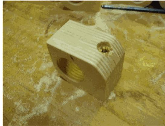
A tube clamp, with the brass insert for the hand clamp knob installed. On the backside of the clamp, two other brass inserts are installed to allow the clamp to be mounted to the secondary ring face.
