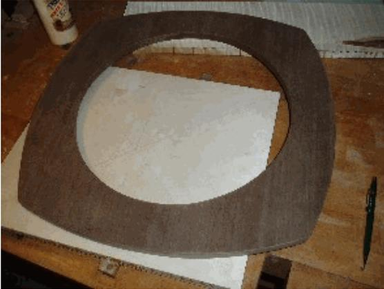
holes in the secondary ring to permit the truss tubes to pass all the way through the secondary ring. I figured this would allow the use of a binoviewer more easily in the field (by just sliding the secondary closer to the primary using the same trusses).
