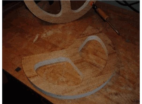
first Dob construction; the altitude bearing could have easily been made at 180 degrees. If I were to do it again, I would make this bearing the more conventional semicircle. This photo shows the bearings prior to sanding and finishing.
