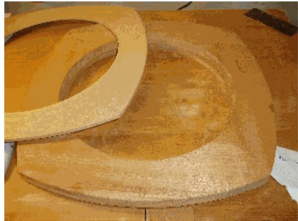
A template for the mirror box endcaps is made from 1/4" hardboard. This template provides a consistent form for making the top and bottom endcaps. The template is applied to the rough cut endcap using hot glue or double-sided tape. Then a router with a flush trim bit is used to smoothly cut the end cap to the exact shape of the template.
