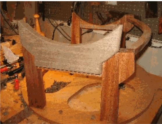
The extension block was fabricated from thick walnut to match the mirror box tube. The outlines of the mirror box were traced and laid out on the extension block. The block was rough cut on the bandsaw. A rabbet was cut by hand using saw and bench chisels. The extension was then fitted and glued to the rocker box. This block successfully raised the scope closer to eye level, and also provided clearance for the truss tubes to avoid the front stretcher tenon.
