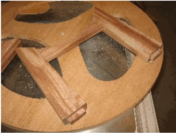
The base of the rocker box is fabricated from 1/2" Baltic birch, cut on the circle jig and with several holes cut out to save weight. It is not essential that this piece be extremely rigid, because it is later reinforced by the mortise and tenon design of the rocker box. The sides of the rocker box are made from solid mahogany and joined with strong mortise and tenon joinery. Note how the top of the rocker box is curved to match the altitude bearings.
