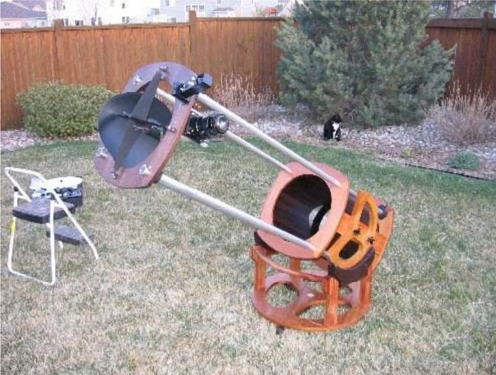
12" f5 lightweight Dobsonian telescope, constructed primarily from mahogany and Peruvian walnut hardwoods. The bottom mirror box employs a lightweight coopered tube, and the entire scope weighs approximately 55 lbs.
