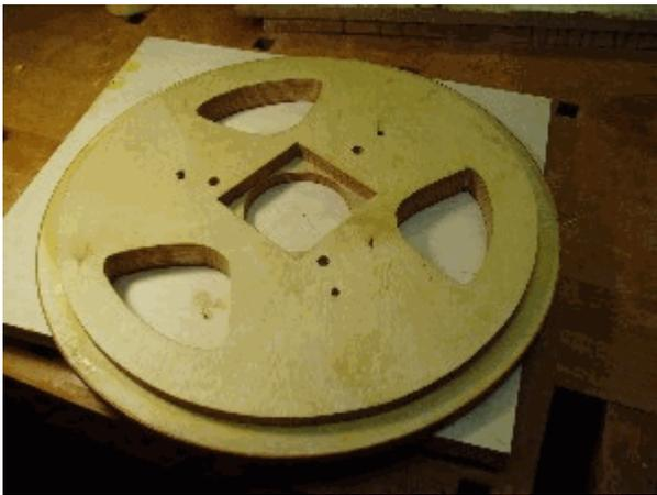
The rough cut cell mounting plate. The mounting plate is made from two sheets of glued 1/2" Baltic birch. The sheets were then cut using the circle cutting jig. The edges were rabbeted with a router, and cutouts were added for the fan and for holes to improve air circulation. Note the three sets of drilled holes, which are later used for the push-pull bolts for adjusting the mirror cell.
