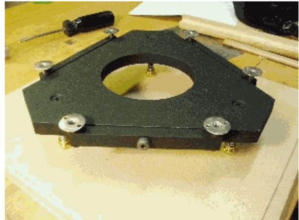
The mirror cell, assembled and painted. Note the six threaded flange inserts, which are elevated appx 1/4" above the main plate. These six inserts form the support points for adhering the mirror. The cell is adhered to the mirror back using silicone RTV (spacers are used to maintain a thickness of about 1/16" of RTV ).
