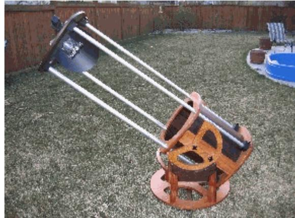
Here is the scope, set up for some backyard viewing. Shown is my heaviest eyepiece (a large Zeiss 30mm 75° eyepiece from military surplus, via Markus Ludes in Germany). The scope is slightly backside heavy, and when using lighter eyepieces, I add some frontside counterweights (large knurled steel nuts that fit ideally in the inside of the truss openings).
