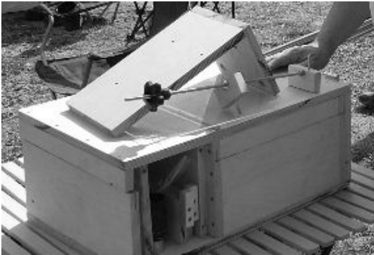
The Scope-In-A-Box packs an equatorially-mounted 12 inch Newtonian for airline carry-on, by Tom Edgar of Laramie.
