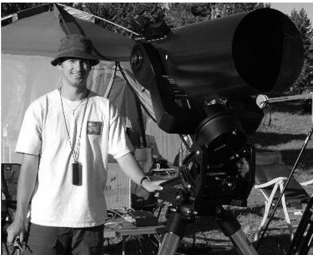
Max Moe imaged a 15 th magnitude asteroid for over 7 hours with his 12 inch SCT to detect its rotation.
